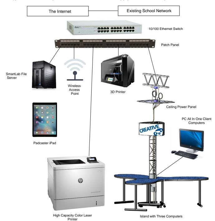
The Island distributes Ethernet and Power Connections from the Ceiling Power Panel to outlets that computers plug into.
